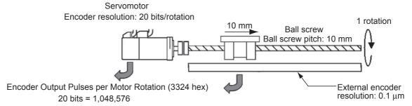
External Encoder Output Pulse per Motor Rotation (3325 hex) 10 [mm]/0.1 [ $\mu$ m/pulse] = 100,000 [pulses]
