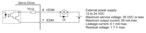
Di: Surge voltage prevention diode (Use a high-speed diode.)
