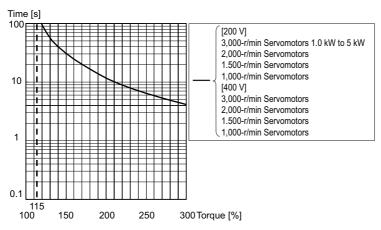
When the torque command = 0, and a constant torque command is continuously applied after 3 or more times the overload time constant has elapsed, the overload time t [s] is
