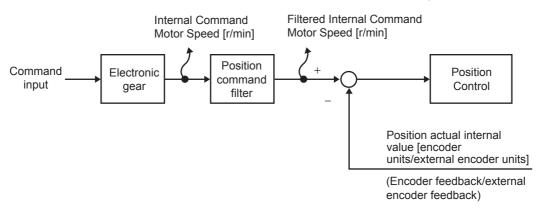
\*2 The position error is calculated for the command input after processing for the position command filter. The pulse position error or fully-closed position error is reversely converted to command units for application. The pulse position error or fully-closed error is the error for the position control input.
