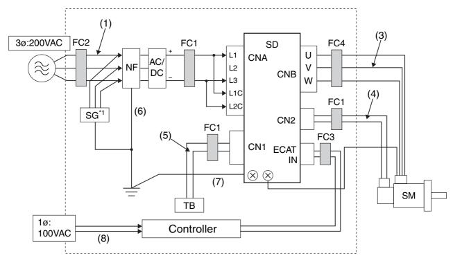
Note L1 and L3 are the main circuit power supply input terminals. Connect the positive wire to L1 and the negative wire to L3.
