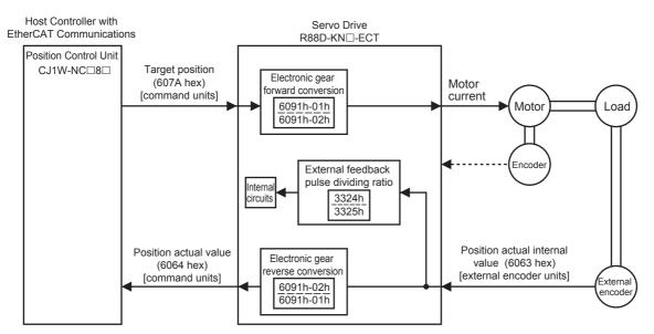
**Note** The electronic gear function is not supported for unit version 2.0. For the Servo Drives with unit version 2.0, set the electronic gear ratio to 1.1.
