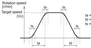
ta = Vc / Maximum motor rotation speed × 3312 hex × 1 ms td = Vc / Maximum motor rotation speed × 3313 hex × 1 ms ts = 3314 hex × 1 ms
