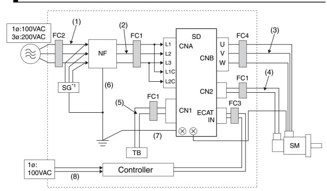
\*1 Not required for single-phase models with a 100-VAC input.
