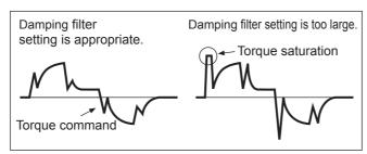
When setting the damping frequencies, reduce the setting if the torque become saturated and increase the setting to make operation faster. Normally 0 is set.
