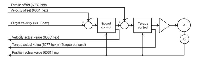
The following diagram shows the control function configuration of the Cyclic synchronous velocity mode.
