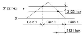
• The settings for the Gain Switching Level in Speed Control (3122 hex) and the Gain Switching Hysteresis in Speed Control (3123 hex) are enabled absolute values (positive/negative).
