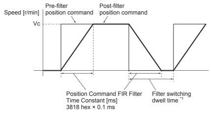
\*1 Change the setting on 3818 hex only after you stop the command pulse and the filter switching dwell time elapses. The dwell time is calculated by the following formulas depending on the value set on 3818 hex. If 3818 hex set value ≤ 10 ms, the set value × 0.1 ms + 0.25 ms. If 3818 hex set value > 10 ms, the set value × 0.1 ms × 1.05.
