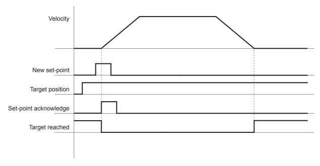
The Target value can be changed while PTP positioning is in progress.
