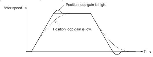
• If the speed loop gain and position loop gain are optimally set, the motor operation for the command delays 2/Kp at acceleration and delays 3/Kp at deceleration.
