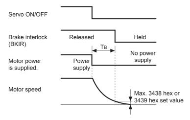
The time  $T_B$  in above drawing is either the brake timing during operation (i.e., the set value  $\times$  1 ms) or the time taken until it goes below the value set in the Brake Threshold Speed During Operation (3439 hex), whichever is shorter.
