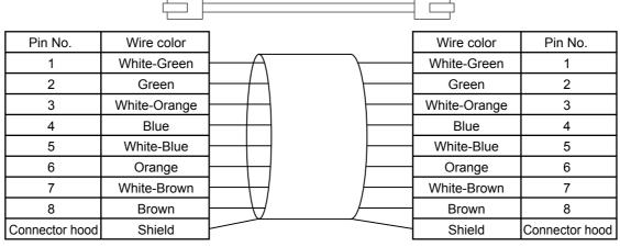
Note 1 Connect the cable shield to the connector hood at both ends of the cable.
