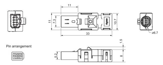
**Note** The recommended cable is a 6-core shielded cable with a wire size of AWG30 to AWG26 and a finished outer diameter of 6.7 mm or less.
