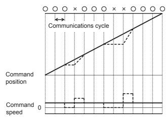
Solid line: Command compensation enabled. Dashed line: Command compensation disabled.
