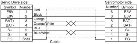
[Servo Drive side connector] Connector model 55100-0670 (Molex Japan) AWG22×2C + AWG24×2P UL20276 (3~20m) AWG16×2C + AWG26×2P UL20276 (30~50m)
