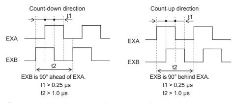
\*3 For the external encoder connection direction, set the direction so that count-up occurs when the motor shaft is rotating in the CCW direction, and count-down occurs when the motor shaft is rotating in the CW direction. If the connection direction cannot be selected due to installation conditions, the count direction can be reversed using External Feedback Pulse Direction Switching (3326 hex).
