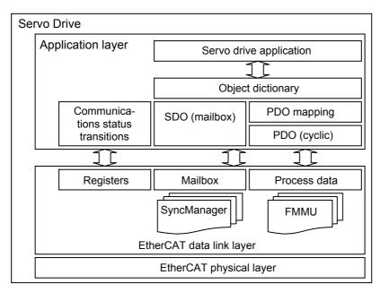
Normally, multiple protocols can be transmitted using EtherCAT. The IEC 61800-7 (CiA 402) drive profile is used for G5-series Servo Drives with Built-in EtherCAT Communications.
