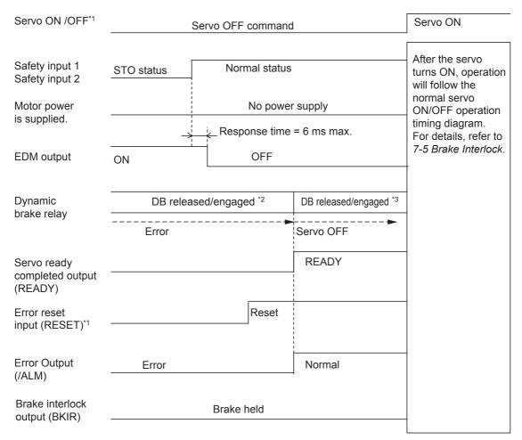
Make sure that servo ON input is turned OFF when you return the input signals of safety inputs 1 and 2 to ON. If an error exists in this state, be sure to clear the error when both safety inputs 1 and 2 have returned to ON state. Also, depending on the execution timing, an Other Error (Error No. 99.9) may occur. If this error (Error No. 99.9) occurs, turn OFF and then ON the power again.
