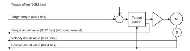
The following diagram shows the configuration of the Cyclic synchronous torque mode.
