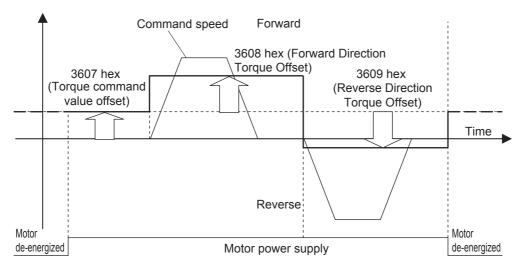
The Torque Command Value Offset (3607 hex) reduces the variations of positioning operations due to the movement directions when a certain amount of unbalanced load torque is always applied to the motor at the vertical axis by setting the torque command.
