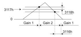
• The settings for the Gain Switching Level in Position Control (3117 hex) and the Gain Switching Hysteresis in Position Control (3118 hex) are enabled as absolute values (positive/negative).
