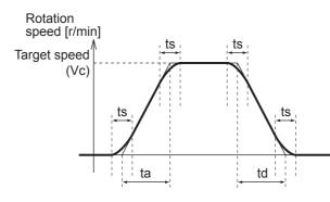
ta = Vc / Maximum motor rotation speed × 3312 hex × 1 ms td = Vc / Maximum motor rotation speed × 3313 hex × 1 ms ts = 3314 hex × 1 ms
