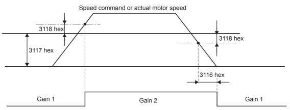
Note The "speed command" is the Motor Control Effort (401A hex) [r/min].
