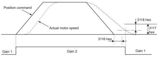
Note Whether there is a position command is determined by changes in the Target position (607A hex).
