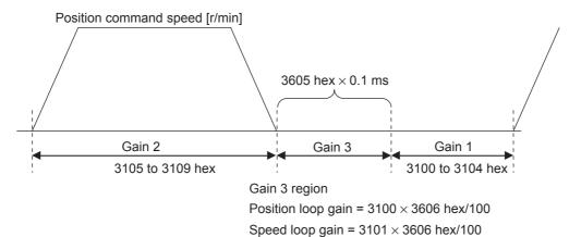
The gain 1 values are used for the speed loop integral time constant, speed feedback filter time constant, and torque command filter time constant.
