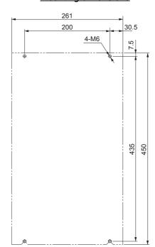
3-phase 400 VAC: R88D-KN06F-ECT/-KN10F-ECT (600 W to 1.0 kW) 3-phase 400 VAC: R88D-KN15F-ECT (1.5 kW)
