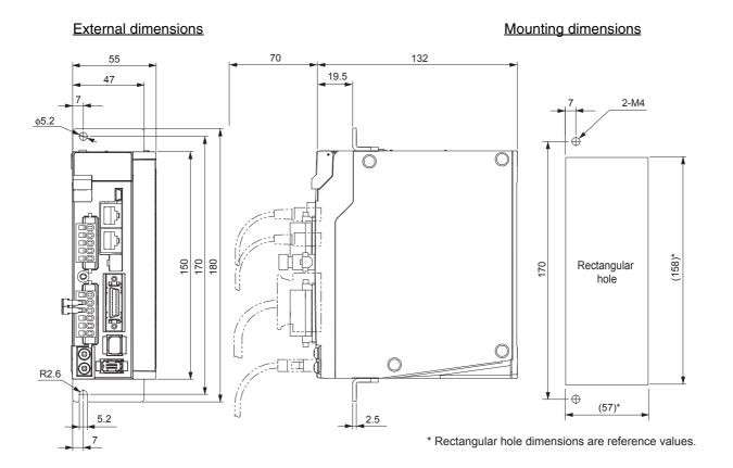
Single-phase/3-phase 100 VAC: R88D-KN04L-ECT (400 W) Single-phase/3-phase 200 VAC: R88D-KN08H-ECT (750 W)
