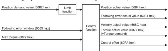
The following diagram shows the control function configuration of Profile position mode.
