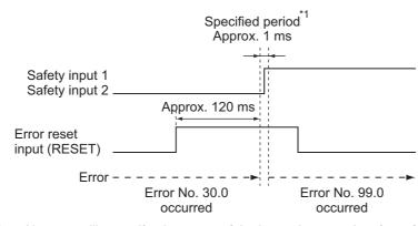
\*1 Error No. 99.0 will occur if at least one of the input photocouplers for safety inputs 1 and 2 is turned from OFF to ON.
