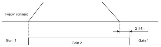
Note Whether there is a position command is determined by changes in the Target position (607A hex).
