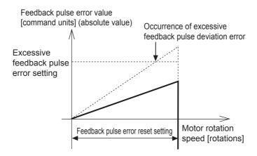
• Ensure that an appropriate value is set to the Hybrid Following Error Counter Reset (3329 hex), before you use the feedback pulse error counter reset. When the set value is extremely small, the protective function may not work to prevent any erroneous operation due to improper connection of the external encoder.
