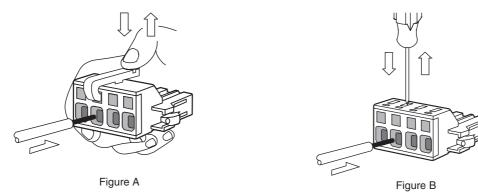
4 With the wire insertion slot held open, insert the end of the wire.
