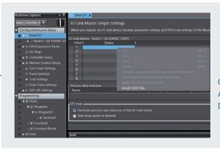
You can set IO-Link device information that can be easily obtained from the physical system configuration. Maintenance is possible even if connected sensor information is unknown.
