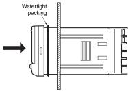
Insert the fixture into the grooves on the left and right sides of the rear case and push until it reaches the panel and is fixed in place.
