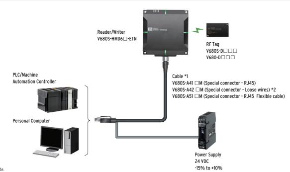
The cable can be extended up to 60 m by using the Extension Cable V680S-A40  $\square$ M (cable length: 10/20/50 m) or V680S-A50  $\square$ M (Flexible cable, cable length: 2/10/20m).
