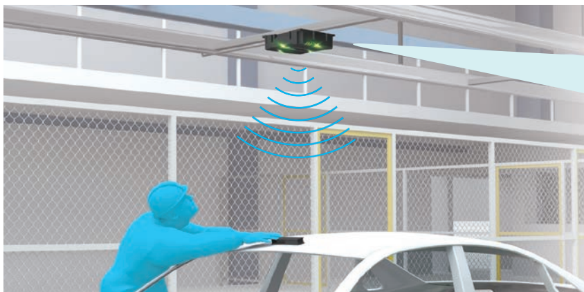
Check the reception level with the indicators on the reader/writer to find the best installation position of an RF tag
