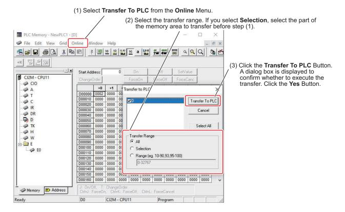
This transfers data from the computer's data memory (DM) to the PLC. In the same way, transfer the PLC memory data that you created during preparation, except for data in the DM Area.
