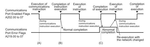
To switch the network, the destination network information in the control data for each communications instruction (SEND, RECV, or CMND) is changed to that of the other destination network, as shown below.
