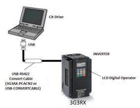
**3.** Use the CX-Drive autodetect hunction in order to go online with the 3G3RX inverter:
