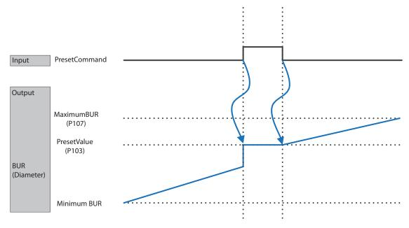
BUR = Build Up Ratio (Diameter Ratio)
