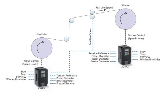
**Note:** In this specific Winder/Unwinder Application program, the tension set point is given through the analog input O2 and the real line speed through the analog input O.
