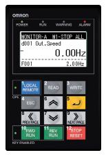
Note: It is recommended to use option 02: rotate autotuning. Please, be sure that the shaft is free (no gear/run connected).
