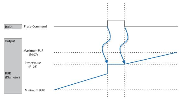
BUR = Build Up Ratio (Diameter Ratio)
