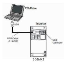
**3.** Use the CX-Drive autodetect 4 function in order to go online with the 3G3RX/3G3MX2 inverter:
