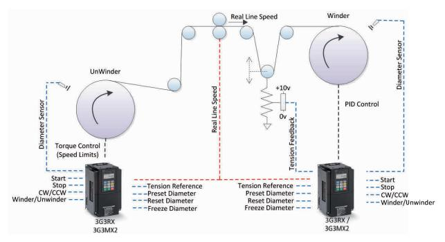
Note: In this specific Winder/Unwinder Application program, the diameter sensor is given through the analog input O2 (RX)/OI (MX2) and the tension feedback through analog input O. Winder line speed reference must be given through communications.
