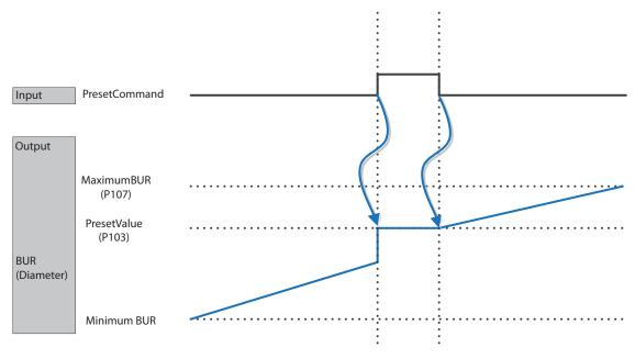
BUR = Build Up Ratio (Diameter Ratio)
