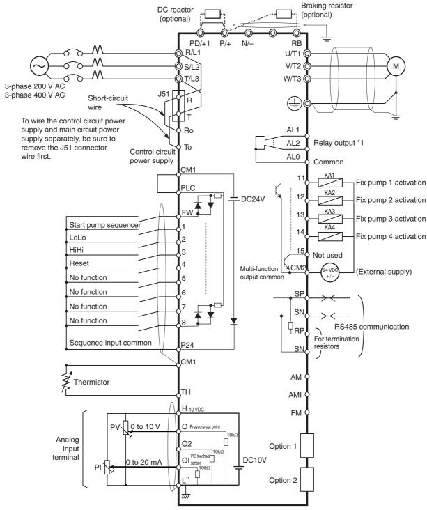
$^{\ast 1}$  L is the common reference for analog input and also for analog output.
