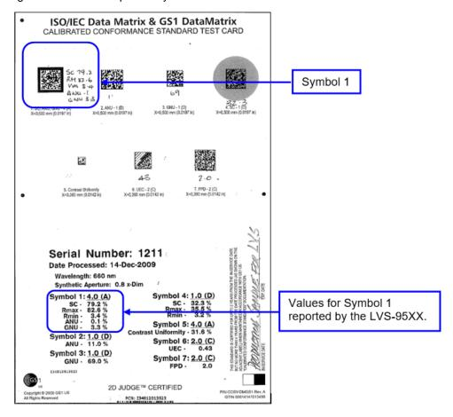
If the results do not match the CCSTC, recalibrate the LVS-95XX and check the results of the calibration on the calibration card measurements. Contact Omron Microscan technical support if the results do not match.
