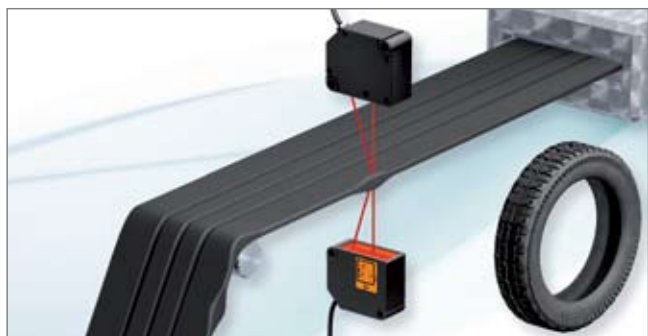
▲ Black rubber thickness inspection
