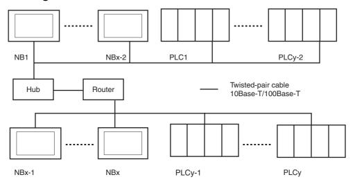
ъ 5 X represents the amount of NB / NB-S series products, and y represents the amount of PLC. The relationship between x and y must meet the following conditions:
