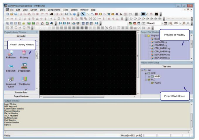
The Project Library Window contains: Connector, PT, PLC, Parts, Function Parts and Project Database.
