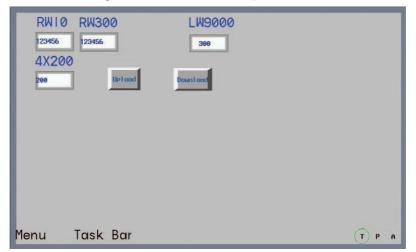
Perform the offline test, change LW9000 to 300 and input "123456" to RWI0, as shown below:
