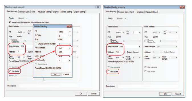
The settings of Number Input components NI2 to NI4 are the same as that of NI1, and their addresses are LW10, LW20 and LW40 respectively.
