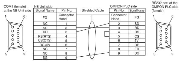
The cable for connecting the NB7W Unit serial port COM1 to OMRON NX1W-CIF01 (RS-232C)
