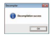
The prerequisite for the decompile operation is "Allow Decompilation" is checked and the password is set in the [PT Extended Properties] tab during the project creation. The default decompilation password is 888888.
