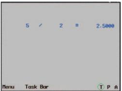
Now the basic specification is completed. However, the Macro still have a problem. When entering "0" into LW1 and executing the Macro, an error occurs and the error can affect the normal operation of the system. In this case, a check should be entered into the operand.
