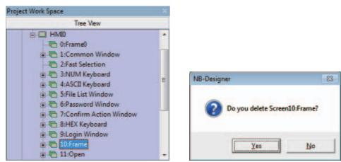
**Note** Frame 0, Frame 1 to Frame 9 are all the default screens for the system, and they are not allowed to be deleted.
