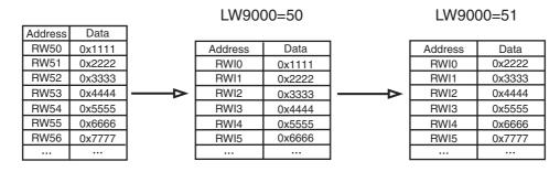
For example, we specify one project and select [MODBUS RTU] as the PLC Type in system parameters. The function of transferring the 5-word text beginning from address 200 with the address type of 4X to the address of recipe memory (RW300) is as shown below:
