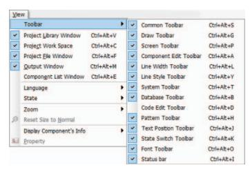
The options in the [View] menu are used to control the various kinds of toolbars to be displayed or not.
