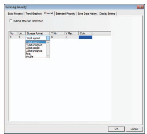
**3** Switch to the [Channel] tab and set the parameters related to each track line.
