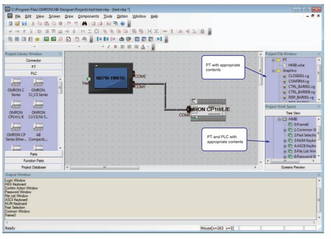
Once the PLC and PT are dragged in, the "Project File Window" and "Project Work Space" will be filled with appropriate content, as shown below:
