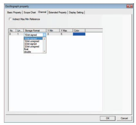
**3** Switch to the [Channel] tab and set the parameters related to each graph.
