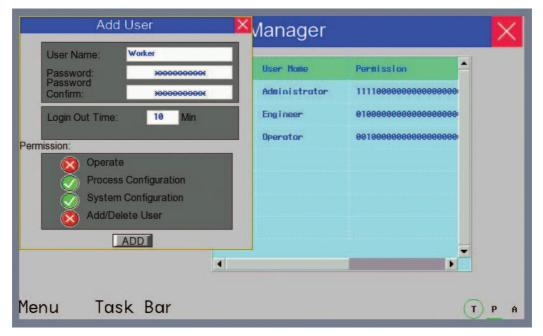
Input the User Name to be added, set the Password and the Password Confirm, and then set the Logout Time for this user and assign the Permission. After the setting, click "ADD" to complete "Add User" operation.
