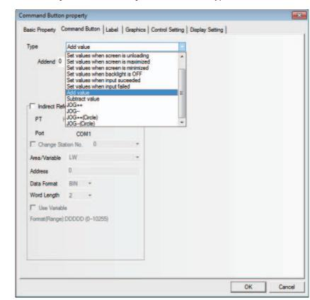
2 Switch to the [Command Button] tab and set the "Type" for the Command Button component.
