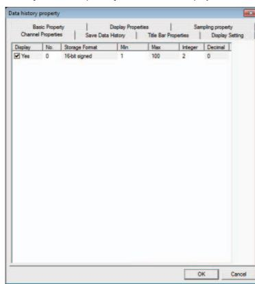
**4** Switch to the [Channel Properties] tab and set the display information for each channel.
