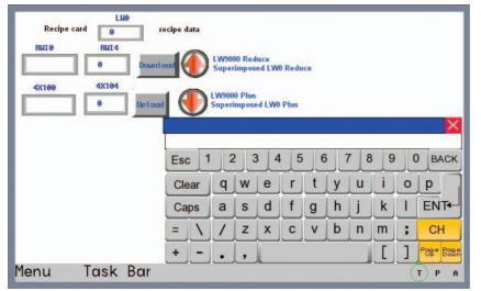
Input the 10 groups of recipe data into the recipe memory one by one, then switch to Group 8 of recipe data to change the name to "KKKKKKK", recipe data to "1234", then you will see the data in 4X100 and 4X104 will become "KKKKKKK" and "1234" respectively after the Download button is pressed, as shown below:
