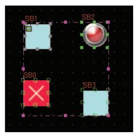
When the user selects the multiple components including the locked component to perform the operation of movement etc, this locked component will have no response to this operation. Please note that there will be one lock-shape mark on its original icon, as shown above.
