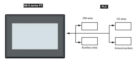
NB-S series PTs can be connected to the PLC manufactured by OMRON using the Host Link method.
