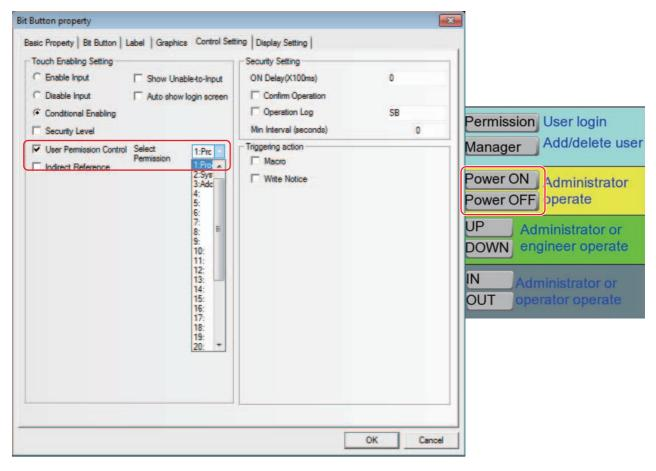
Setting "Use Permission Control" for the component means only the user having this operation authority can operate the component restricted by this authority.
