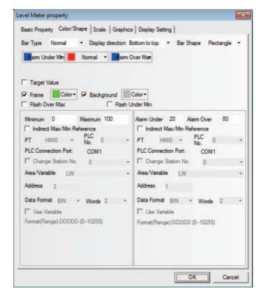
2 Switch to the [Color/Shape] tab and make settings as shown below.
