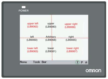
For each area, there is/are one or more address bit(s) corresponding to it. When the Text Input or Number Input in the screen is triggered, the corresponding address bit(s) will be turned ON.
