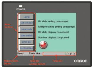
In the task bar, 16 icons can be arranged at the same time. The functions keys of [Minimize] or [Title Bar in Pop-up Screen] included in Pop-up Screen allow the screens to minimize in the task bar. For details, refer to *3-7-2 Function Key (Page 3-201)* in *NB-Designer Operation*.
