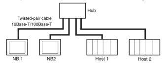
The UDP communication for NB / NB-S series products is only limited the local network, but the Ethernet communication crossing the network segment is allowable with the prerequisite of using the router. That's to say, the supported network is only limited to the local network, but the various devices in the network can cross the network segment. Please take the following architecture as reference.
