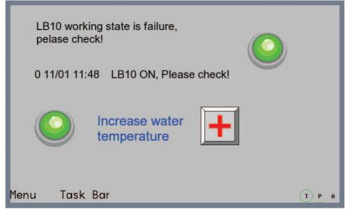
When LB10 or LW30 is triggered for its corresponding triggering conditions is satisfied, the related event information will be displayed. The popup screen 4 and screen 5 for the 2 events registered in the [Event Setting] are the pop-up screens to be ejected when the event is triggered.
