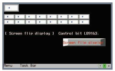
Method 2: The flipping of the screen is controlled by the local special memory LB9163 (LB9163 is read/write type.). When LB9613 is turned ON, the screen is displayed vertically-flipped. When the flipped screen display function is controlled by LB9163, the flipping function can't be maintained after the power failure or restart of the screen.
