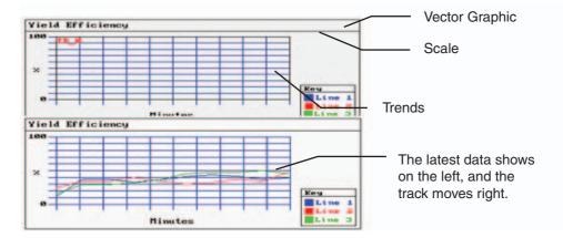
A typical example of Data Log is as above shown. Use one Vector Graphics as background, and use the Scale component to express the information on the related Data Logs. Then place the Data Log component above the Vector Graphics.
