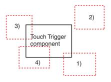
1), 3) and 4) locate in the valid triggering area, while 2) locates in the invalid triggering area.
