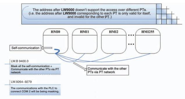
Taking an example the case using masking function for HMI0, the corresponding of LW memory and masking object is displayed as below.
