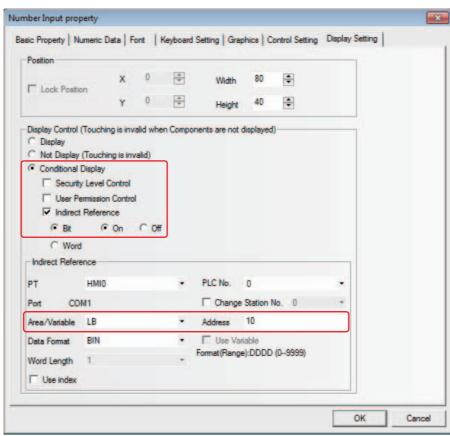
Perform the offline test. When LB10 is Off, the number input component is hidden, as shown in the following left graphics.
