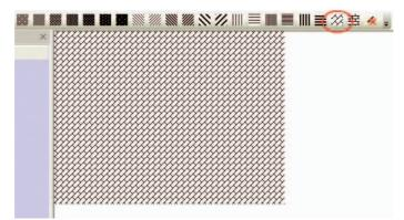
In order to add fill effect to the shapes, select the shape to add fill effect and select the fill effect. The procedure to set the fill effect is the same as the one for adding fill effect to the PT. But when setting the fill effect to the components, [Pattern Color] is applied to the outline color and [Background color] is applied to the component's color. The parameters set to the shape is reflected as below.
