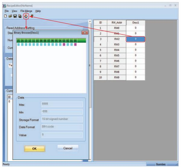
In this case, the value of RW2 is 9, and bit addresses of 03 and 00 indicate the status of ON in binary browser.
