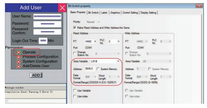
Add User Operation Confirmation: Place one Bit Button component with the address of LW9167 and switch type of "Set" for confirming the added user permission.
