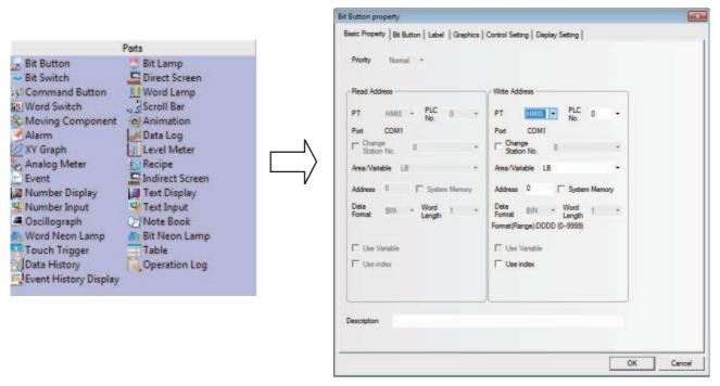
After the various Properties of this component are set, click the [OK] button. And you can see this component has been placed in the screen after exiting from this dialog box. If required, you can adjust the size of the component by changing settings in "Position" in "Display Setting" tab or drag it to the desired position.
