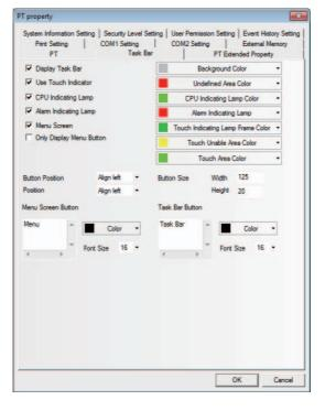
**Note** The Menu Screen is displayed on the left side or the right side of the panel during the operation. In edit window state, the Menu Screen is an independent screen, and it is Frame 2 by default. For details, refer to *3*-10-2 Task Bar (Page 3-294) in NB-Designer Operation.
