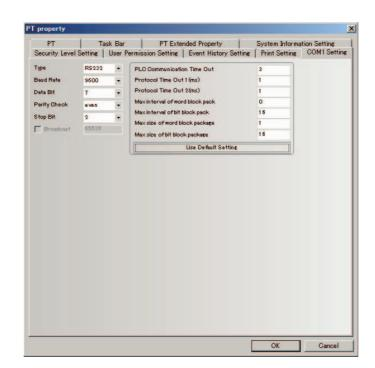
There are [COM1 Setting] here because NB Unit has 1 serial port. You can make the connection to 1 PLC through this serial port.
