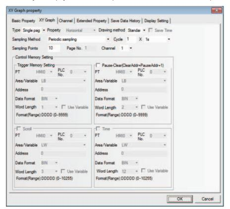
**2** Go to the [XY Graph] tab and set the parameters related to the XY Graph.
