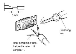
4 Pull the heat shrinkable tubes back to the soldering parts, heat them with a heat shrinking gun to make them shrink.
