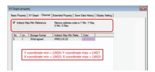
Example: When the maximum value and minimum value of a line graph (Drawing method: Track) are specified indirectly.
