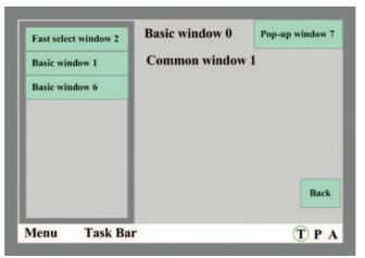
(14)Pressing [Common Sheet 1/6] can realized the switching among the Common Sheet.
