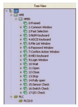
All the components contained in each screen will be displayed here, and if there is no component in a screen, nothing will appear below it.
