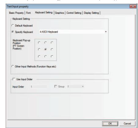
**3** Switch to the [Keyboard Setting] tab and select the keyboard type.
