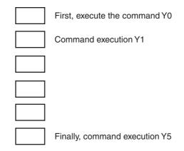
The control process is as follows: Y0 ON/OFF $\rightarrow$ Y1 ON/OFF (Step 2)  $\rightarrow$ Y2 ON/OFF (Step 3), ...,  $\rightarrow$ Y5 ON/OFF (Step 6).
