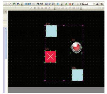
Resize the multiple components simultaneously dragging by mouse each point on the corners. Above, the selected area is pink.
