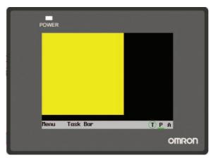
Press the function key and pop-up Frame 10 will cover the function key, which is caused by the transparency of 0% for Frame 10, as shown below.
