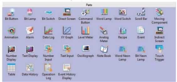
When a project is created, and the Edit Window is entered, it just needs to drag the required components to the Edit Window.
