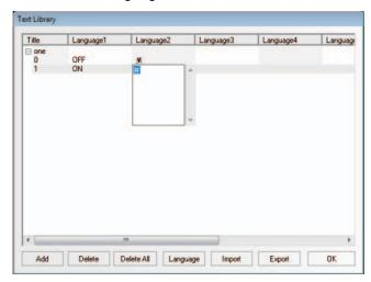
(5) If you use 2 states, it just needs to input the corresponding text to state 0 and state 1 respectively for each language, and then click "OK" after the completion of the text addition.
