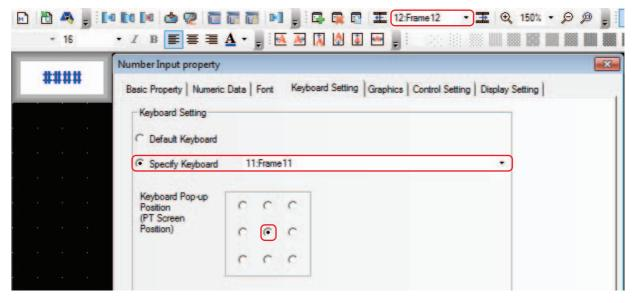
(6) Perform the offline test and click the Number Input component to make the keyboard pop up, as shown below:
