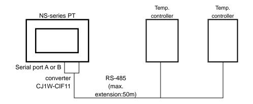
By using another communications port, you can simultaneously connect temperature controllers and a host. With one more serial port, NS can connect PLC, barcode reader, Memory Link and can communicate with CX-Designer.
