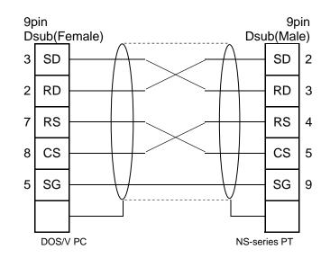
Above wiring is identical with the NS to and from CX-Designer wiring.
