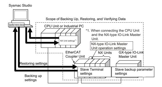
The range of data that is backed up is different for GX-type IO-Link Master Units and NX-type IO-Link Master Units, as described below.
