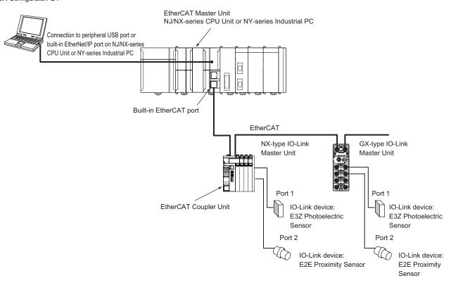
For the above system configuration, use CX-ConfiguratorFDT to create a network configuration as shown below.
