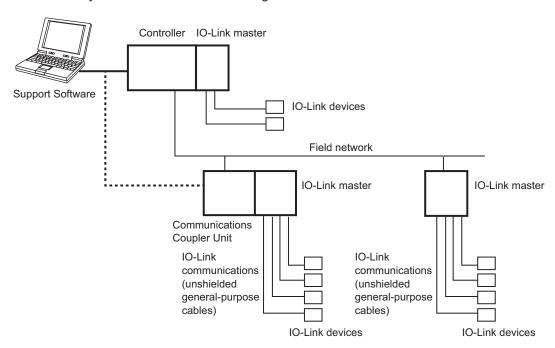
The configuration elements of an IO-Link System that uses an OMRON IO-Link Master Unit are described below.
