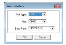
2 Set the **Port Type**, **Port**, and **Baud Rate** to suitable values and then click the **OK** Button to connect to the CJ2-series PLC. If the connection is successful, the **Browse Network** Dialog Box is displayed.
