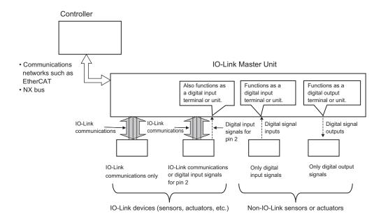
The above types of data exchange are set in advance with the communications mode parameters in the OMRON IO-Link Master Unit. Refer to *1-4 Communications for IO-Link Systems* on page 1-15 and *2-2-1 In IO-Link Mode* on page 2-5.
