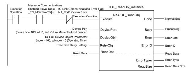
\*1. Use this when you connect the IO-Link Master Unit to a Communications Coupler Unit. This is not necessary when you connect the IO-Link Master Unit to a CPU Unit.
