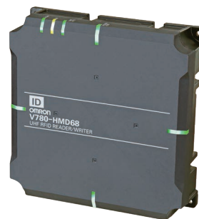
Reads data from RF tag (or writes data to RF tag)
