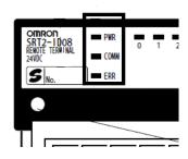
[SRT2-ID08 front panel LEDs]
