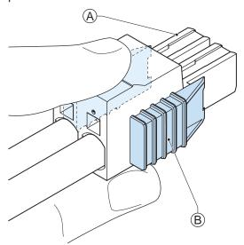
Pushing both orange sliders  $^{\textcircled{B}}$  towards the end of the connector  $^{\textcircled{A}}$  will release the lock when removing the connector.
