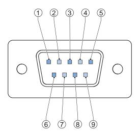
The pin layout represents the RS-232C connector on the IPC.
