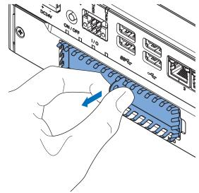
4 Insert the drive cover in the drive bracket bay 1 and move it down 2 so that it locks in the drive bracket.
