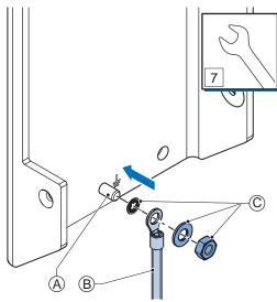
Mount the ground connection wire B to the functional ground terminal A using the washers and nut C. Tighten the nut with a torque of 1.2 N·m max.
