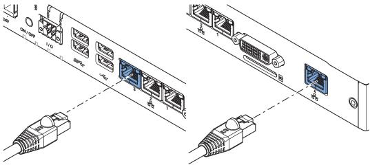
The set of 3 RJ45 Ethernet connectors is available on all models, the single connector is optional.
