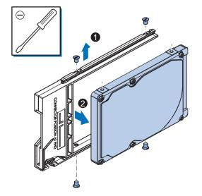
Align the connectors of the replacement drive as shown on the bracket. Then insert the replacement drive in the bracket and insert the 4 mounting screws in the screws with a torque of 0.35 N·m.
