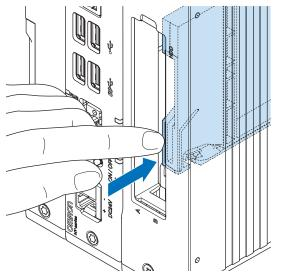
The drive bracket will lock into place when it is fully inserted.
