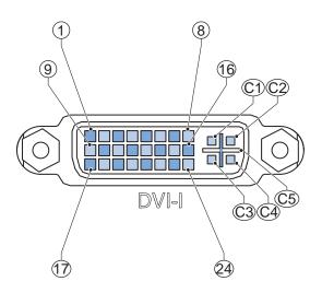
The pin layout represents the DVI-I connector on the IPC Application Controller. Pin numbers increase from left to right for every row.
