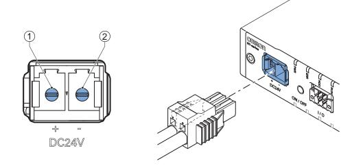
The pin layout represents the power connector on the IPC.
