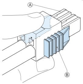
Do not push the orange sliders  $^{(B)}$  in the direction of the IPC because this will unlock the connector.
