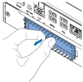
**4** Rotate **1** and then remove **2** the break out part from the drive bracket.
