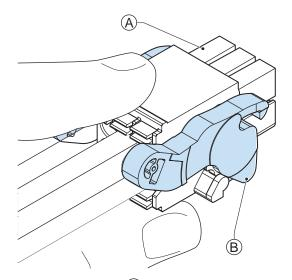
Tilting both levers B will release the I/O connector A from the IPC.
