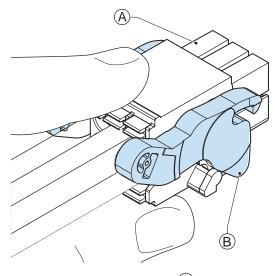
Do not tilt the orange levers  $^{\textcircled{B}}$  because this will unlock the connector.
