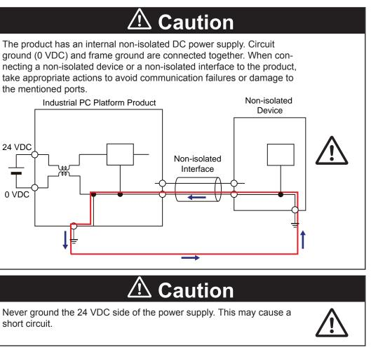
The shielding of the communication connectors are directly bonded to the case and to the functional ground of the IPC.
