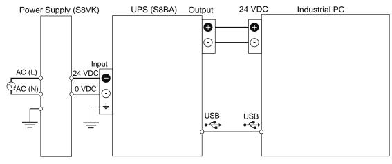
Refer to the UPS S8BA User's Manual (Cat. No. U702) for details. Refer to 5-4-3 Wire the Power Connector on page 5-28 for wiring details.
