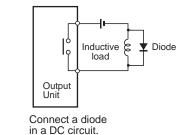
Connect a diode in a DC circuit.
