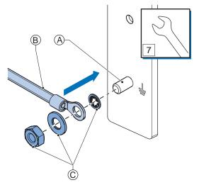
Mount the ground connection wire B to the functional ground terminal A using the washers and nut C. Tighten the nut with a torque of 1.2 N·m max. Refer to 5-3-9 *Wall Mount Procedure* on page 5-20 for wall mounting details.
