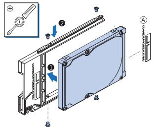
**8** Insert the bracket with the replacement drive into the correct bay of the IPC. Ensure the bracket is completely in the IPC with an extra push.
