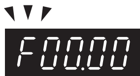
Figure 5.47 Ready for Setting Speed Reference
