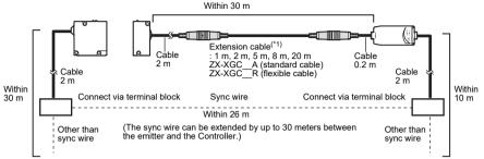
\*1: Up to two extension cables can be connected. However, be sure to limit the total extension cable length between the receiver and the Controller to 30 meters (including the receiver cable).
