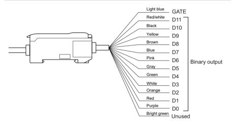
Assignments and Functions of Output Signal Wires p.93
