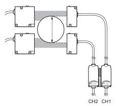
Measurement results can be calculated between two Controllers. Set the expression on the Controller having the larger CH No. The calculation result also is output from the Controller having the larger CH No.
