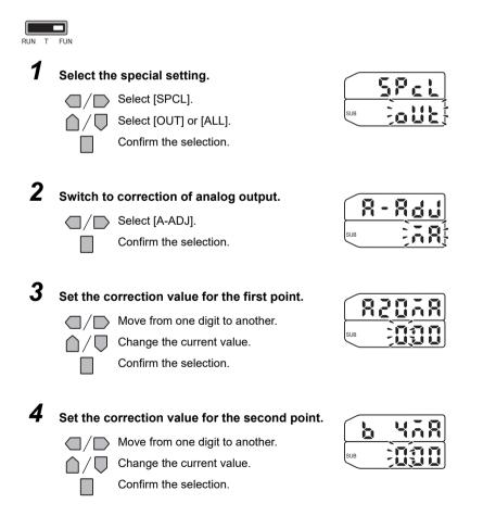
Check that setting of correction values is completed.
