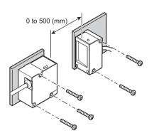
Fix the Sensor onto the mounting base with M4 screws.
