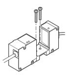
Fix the Sensor onto the mounting base with M3 screws.
