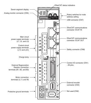
Note: The above picture shows 230 V servo drives models only. The 400 V servo drives have 24 VDC power input terminals for control circuit instead of L1C and L2C terminals.
