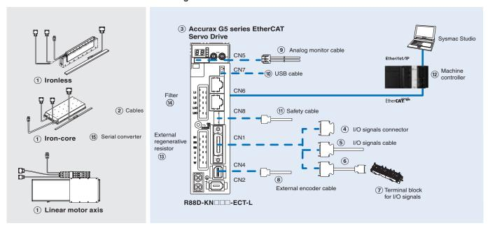
Note: The symbols 12345... show the recommended sequence to select the components in Accurax G5 servo system
