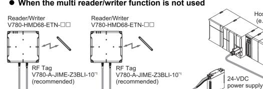
Recommended Power Supply Cable: XS5F-D42□-□80-F (made by OMRON)
