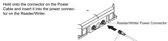
Connector on Power Supply Cable
