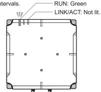
The RUN indicator will light when the Reader/Writer starts in Run Mode.
