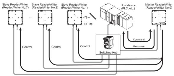
In the Multi-Reader/Writer function, the slave Reader/Writers connected to the master Reader/Writer are differentiated by the following Reader/Writer numbers.
