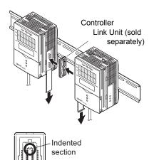
5. Slide the Sensor Controller to insert to the Controller Link Unit connector.
