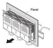
3. Install the small Mount Adapters on the four holes on the Multi-Controller and Sensor Controller.
