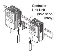
3. Install the cover on the coupler of the controller.
