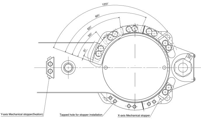
Fig. 3-68 Mechanical stopper positions and movement range (R6YXC700, R6YXC800, R6YXC1000)
