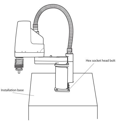
Fig. 3-6 Installing the robot
