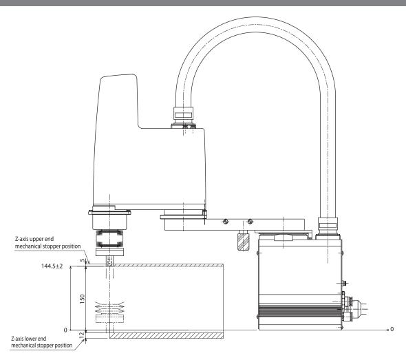
R6YXCH400 (Z-axis mechanical stopper position)
