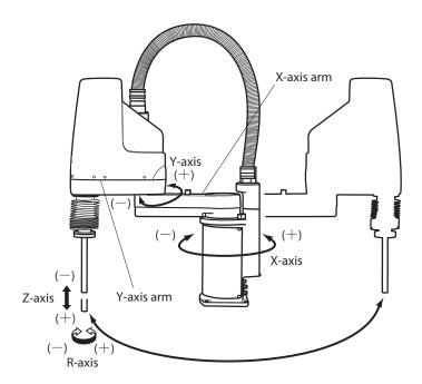
Fig. 2-1 Manipulator movement
