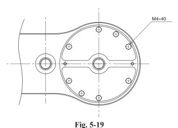
12) Remove the X-axis arm and place it where it will not obstruct the work.
