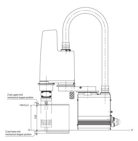
R6YXCH250 (Z-axis mechanical stopper position)
