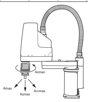
Fig. 3-66 Maximum acceleration on end effector attachment
