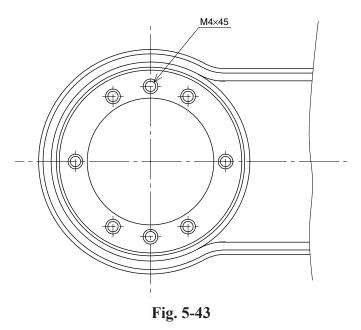
12) Remove the Y-axis harmonic drive from the top of the X-axis arm.
