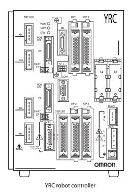
Fig. 2-5 Robot controller
