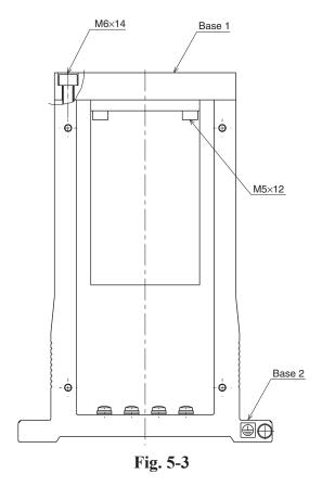
9) Remove the bolts (M5×12L, 4 pieces) securing the motor and remove the motor from base 1. (See Fig. 5-4.)
