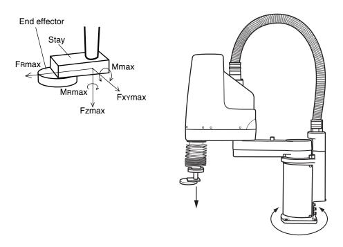
Fig. 3-64 Maximum load applied to end effector attachment
