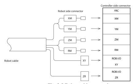
Fig. 3-8 Robot cable connections
