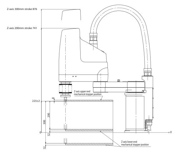
R6YXC500 (Z-axis mechanical stopper position)
