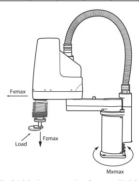
Fig. 3.1 Maximum reaction force applied during operation
