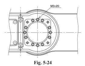
10) Remove the Y-axis arm and place it where it will not obstruct the work.
