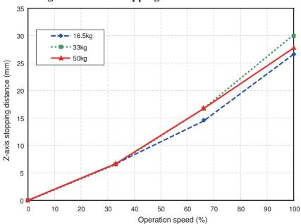
Fig. 3-70 Z-axis stopping distance for R6YXX1200
