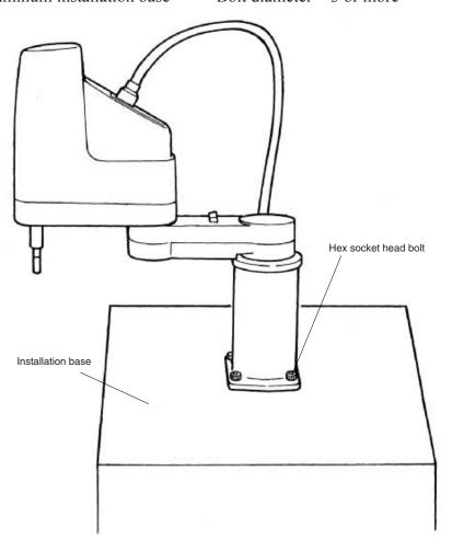
Fig. 3-6 Installing the robot
