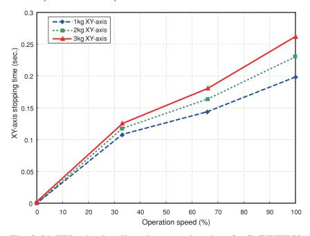
Fig. 3-51 XY-axis plus direction stopping time for R6YXH250
