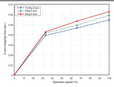
Fig. 3-69 Z-axis stopping time for R6YXX1200
