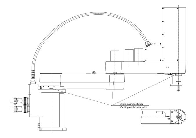
Fig. 4-6 Origin position mark setting example R6YXX1200
