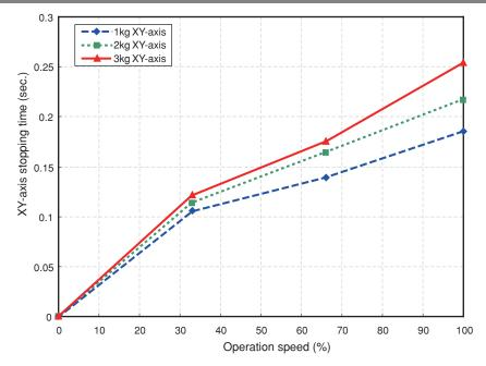
Fig. 3-53 XY-axis minus direction stopping time for R6YXH250
