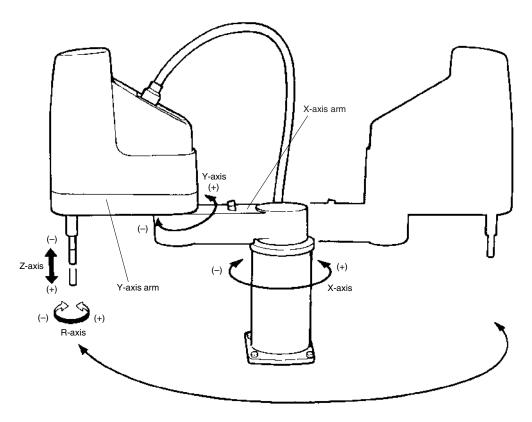
Fig. 2-1 Manipulator movement
