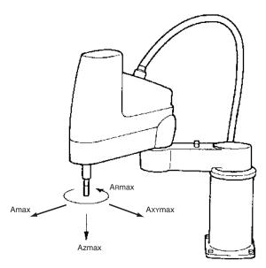
Fig. 3-42 Maximum acceleration on end effector attachment
