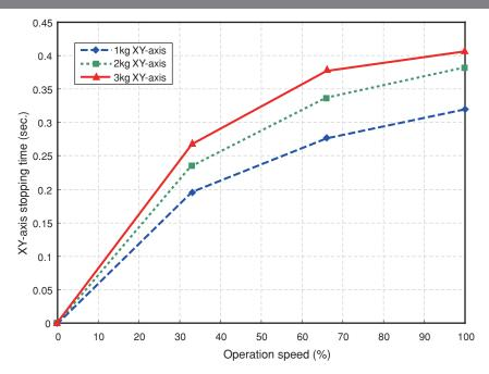
Fig. 3-61 XY-axis minus direction stopping time for R6YXH400
