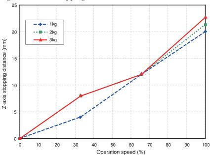
Fig. 3-64 Z-axis stopping distance for R6YXH250 and R6YXH350
