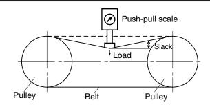
Fig. 4-16 Belt tension adjustment
