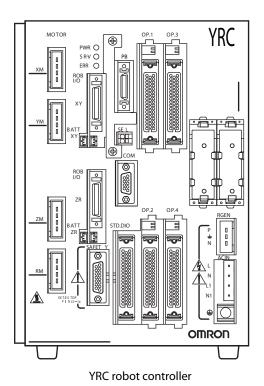
Fig. 2-4 Robot controller
