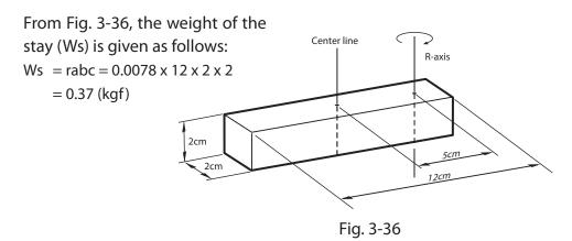
The moment of inertia of the stay (Js) is then calculated from Eq. 3-7.
