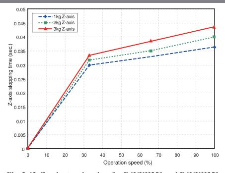
Fig. 3-63  $\,$  Z-axis stopping time for R6YXH250 and R6YXH350
