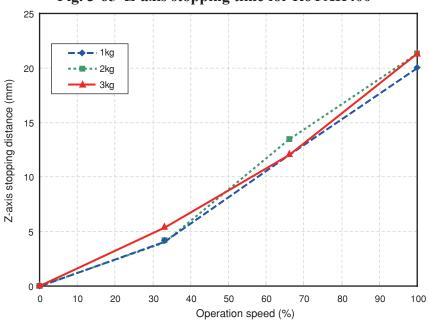
Fig. 3-66 Z-axis stopping distance for R6YXH400
