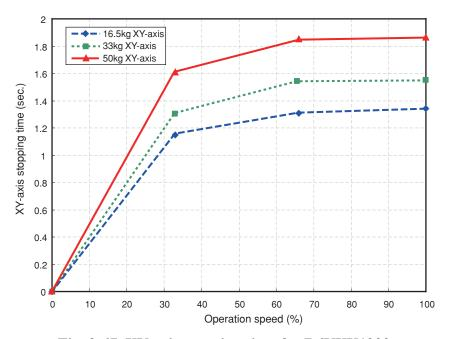
Fig. 3-67 XY-axis stopping time for R6YXX1200
