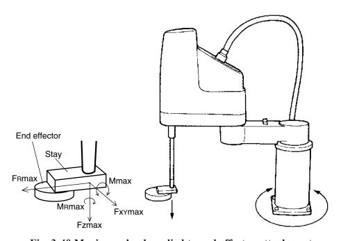
Fig. 3-40 Maximum load applied to end effector attachment
