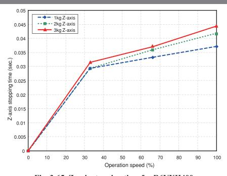
Fig. 3-65 Z-axis stopping time for R6YXH400
