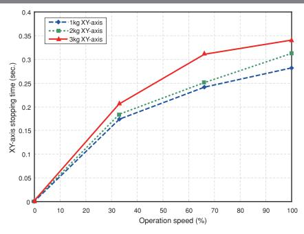
Fig. 3-55 XY-axis plus direction stopping time for R6YXH350
