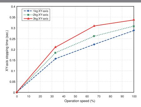
Fig. 3-57 XY-axis minus direction stopping time for R6YXH350
