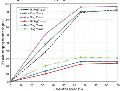
Fig. 3-68 XY-arm stopping rotation angle for R6YXX1200
