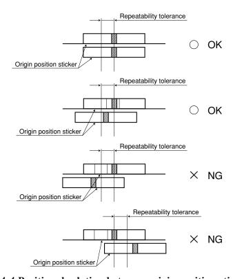
Fig. 4-4 Positional relation between origin position stickers
