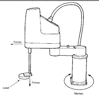
Fig. 3-1 Maximum reaction force applied during operation
