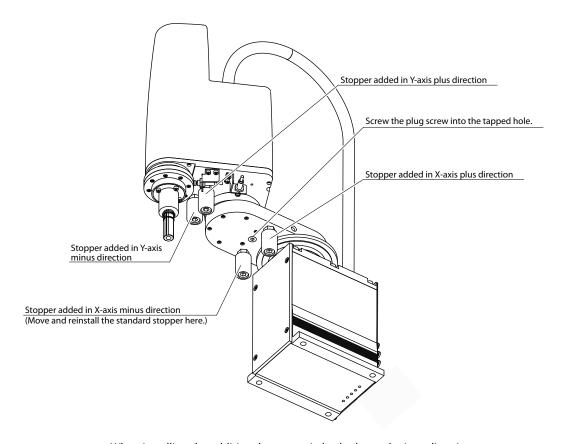
When installing the additional stoppers in both plus and minus directions
