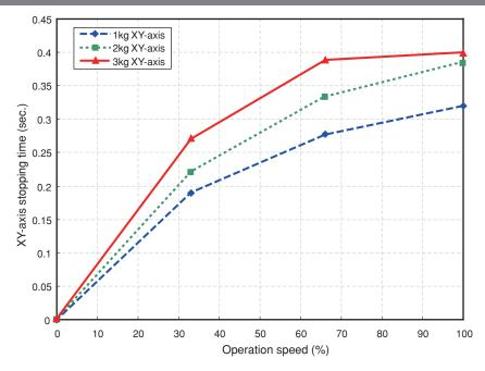
Fig. 3-59 XY-axis plus direction stopping time for R6YXH400
