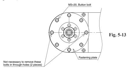
AN O-RING IS FITTED TO THE FASTENING PLATE, SO BE CAREFUL NOT TO LET IT DROP INTO THE PERIPHERAL UNIT. (SEE FIG. 5-14.)
