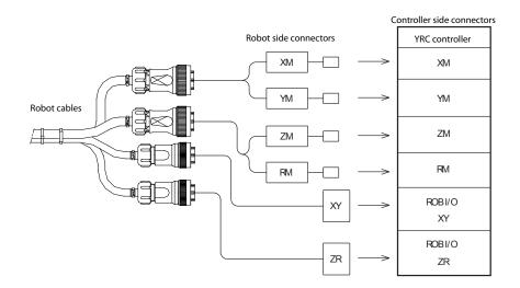
Fig. 3-8 Robot cable connections
