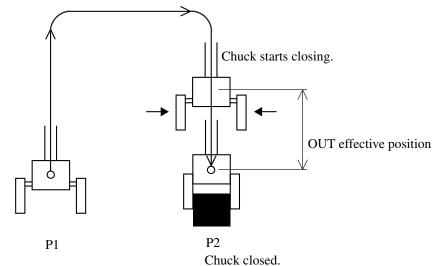
When all of the X, Y, Z and R axes enter the OUT effective position (10000 pulses prior to P2), the chuck starts closing.
