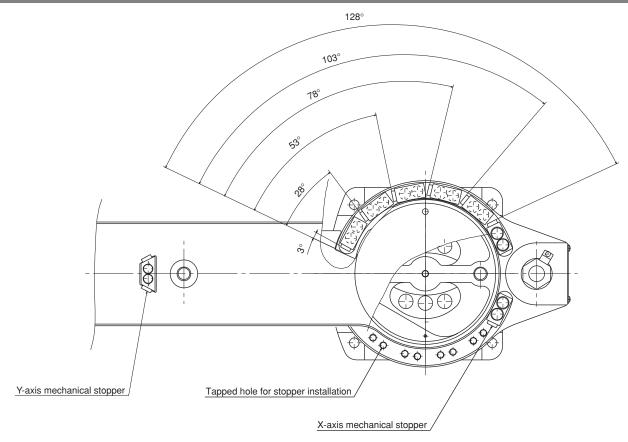
Fig. 3-43 Mechanical stopper positions and movement range (R6YXX1200)
