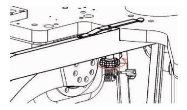
• Now tighten the star nut until the tool is fixed
