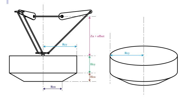
Zu + offset: -760,5 mm Distance from the Z-axis origin position to the tool flange
