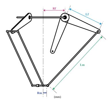
Rf: 200 mm Distance (radius) from the center of the fixed frame to the motor of the axis
