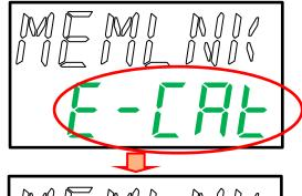
Press the **1 (UP)** Key to change the menu to EIP in blinking.
